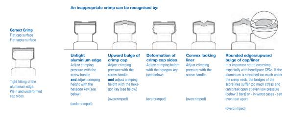
Note that a poor crimp cannot be recognised by simply trying to turn the seal, because PTFE-laminated liners have a very slippery surface, which permits even correctly crimped caps to be rotated if sufficient force is used. Correctly crimped caps can also be turned easily when the liner is in contact with the reduced surface area of a headspace (bevelled top) glass rim.
