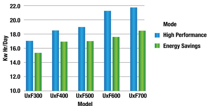
By controlling the temperature and time of the cycles, the energy savings cycle can save up to 15% while still offering tightly-controlled cabinet temperature and excellent door-opening recovery. The high-performance mode maintains the strictest cabinet temperature control.
