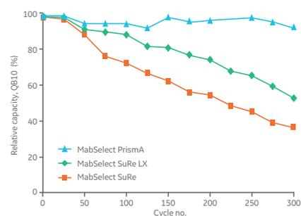
Relative remaining capacity (Q<sub>B10</sub>) for 300 cycles, including CIP with 0.5 M NaOH for 15 min/cycle.
