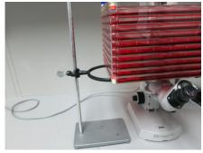
If the microscope stage is not capable of supporting the weight of the Cell Factory system, it is advisable to use an adjustable stand to carry some of the weight of the Cell Factory system.
