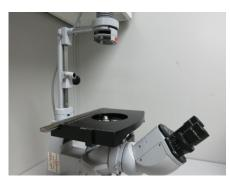
Begin by removing all stage accessories to provide a flat surface for the Cell Factory system to rest upon. If additional space is required, remove the light source.
